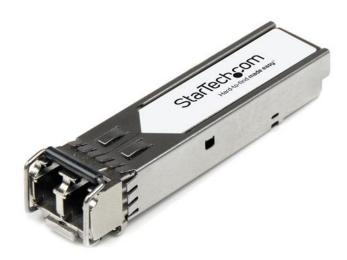
The EG3B0000086-ST is a Citrix EG3B0000086 compatible fiber transceiver module that has been designed, programmed and tested to work with Citrix brand switches and routers. It delivers dependable 1 GbE connectivity over fiber cable, for 1000Base-SX compliant networks, with a maximum distance of up to 550 m (1804 ft).
