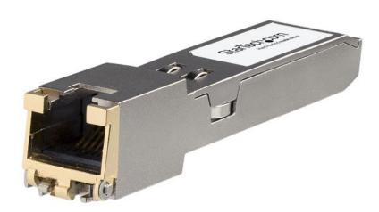
The JL563A-ST is a HP JL563A compatible copper transceiver module that has been designed, programmed and tested to work with HP brand switches and routers. It delivers dependable 10 GbE connectivity over copper cable, for 10/100/1000/10000 compliant networks, with a maximum distance of up to 30 m (98.4 ft).
