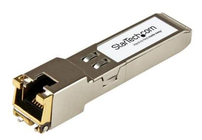
The SFP-TX-ST is a Citrix SFP-TX compatible copper transceiver module that has been designed, programmed and tested to work with Citrix brand switches and routers. It delivers dependable 1 GbE connectivity over copper cable, for 1000Base-T compliant networks, with a maximum distance of up to 100 m (328 ft).
