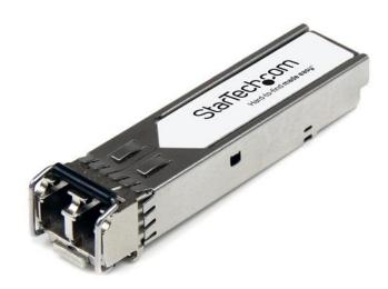
The XG-LR-ST is a Brocade XG-LR compatible fiber transceiver module that has been designed, programmed and tested to work with Brocade brand switches and routers. It delivers dependable 10 GbE connectivity over fiber cable, for 10GBase-LR compliant networks, with a maximum distance of up to 10 km (6.2 mi).
