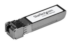
The JD094B-BX60-U-ST is an HP JD094B-BX60-U compatible upstream fiber SFP+ transceiver which pairs with StarTech.com's JD094B-BX60-D-ST. They are designed, programmed and tested to work with 10GBase-BX compatible HP switches and routers. The SFP+ transceiver module supports a maximum distance of up to 60 km (37.3 mi) and delivers dependable 10 GbE connectivity over fiber cabling.
