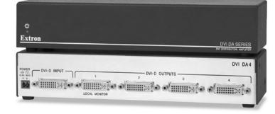
The Extron DVI DA distribution amplifiers with two or four outputs accept a single link DVI input signal and output multiple identical signals to attached devices. These distribution amplifiers provide automatic input cable equalization to ensure optimal image quality on all outputs. The DVI DA distribution amplifiers are ideal for use in all applications that require reliable distribution of high resolution DVI digital video signals.
