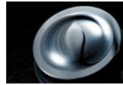
Metal mold for producing the aspherical lens
