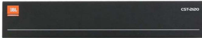
The rack-mountable JBL Commercial® CST-2120 transformer module provides impedance and voltage matching from the CSA-2120 amplifier (with 4 and 8 ohms outputs) to drive 70V and 100V distributed speakers systems. This unit allows the CSA-2120 amplifier without direct 70V or 100V output capability to drive distributed speaker systems designed to operate at those voltages.
