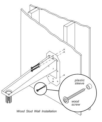
Wall Arms include three wood screws and plastic sleeves (left) for attachment to a wood stud wall. For attachment to a concrete wall additional fastener package ACC 210 must be ordered.
