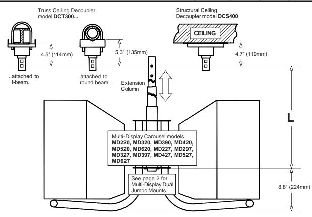
The Extension Column for Multi-Display Mounts is one of three elements required for Multi-Display Ceiling Mount installations. It is available in several lengths which are adjustable at 1" increments (see specifications, above right).
