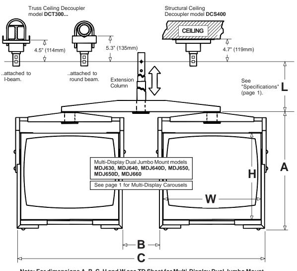
Note: For dimensions A, B, C, H and W see TD Sheet for Multi-Display Dual Jumbo Mount .
