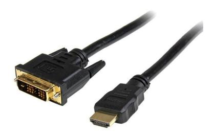
The HDMIDVIMM15 15-foot HDMI® to DVI-D cable enables you to connect a DVI-D video card (or other DVI-D output device) to a display that incorporates HDMI technology; the cable supports bi-directional operation that also allows the reverse configuration, delivering digital video from an HDMI-enabled output to a DVI-D capable display.
