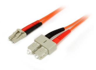
The 50FIBLCSC1 1m LSZH LC to SC Fiber Cable features 50/125 micron fiber for high-speed, high bandwidth data transmissions over Gigabit Ethernet and Fiber Channel networks, with support for duplex multimode applications.
