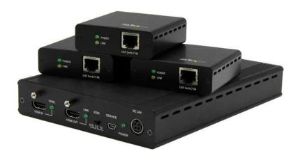
This 3-Port HDBaseT<sup>™</sup> extender kit lets you extend an HDMI® source to three remote locations, using HDBaseT technology. The kit includes three remote receiver units, and the transmitter features a local HDMI output, which gives you the ability to keep a fourth HDMI display at your local video source.
