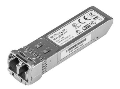
The SFP10GSRST is a TAA compliant Cisco SFP-10G-SR compatible fiber transceiver module that has been designed, programmed and tested to work with Cisco® brand switches and routers. It delivers dependable 10GbE connectivity over fiber cable, for 10GBASE-SR compliant networks, with a maximum distance of up to 300 m (984 ft.).
