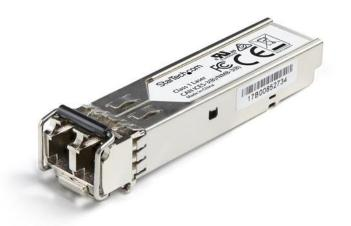
The RX10KMSFPST is a Juniper RX-550M-SFP compatible fiber transceiver module that has been designed, programmed and tested to work with Juniper brand switches and routers. It delivers dependable 1 GbE connectivity over fiber cable, for 1000BASE-LX compliant networks, with a maximum distance of up to 10 km (6.2 mi).
