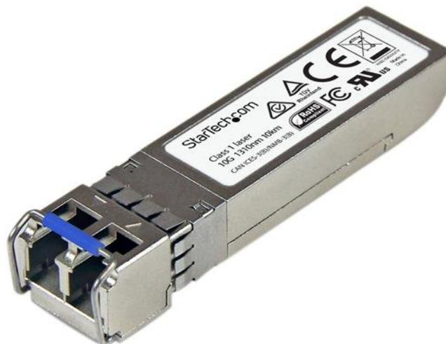
The SFPP10GELRST is a Juniper XBR-000180 compatible fiber transceiver module that has been designed, programmed and tested to work with Juniper brand switches and routers. It delivers dependable 10 GbE connectivity over fiber cable, for 10GBase-LR compliant networks, with a maximum distance of up to 10 km (6.2 mi).
