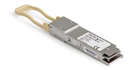
The 40G-QSFP-SR4-ST is a Brocade 40G-QSFP-SR4compatible fiber transceiver module that has been designed, programmed and tested to work with Brocade brand switches and routers. It delivers dependable 40 GbE connectivity over fiber cable, for 40GBase-SR4 compliant networks, with a maximum distance of up to 150 m (492 ft.).
