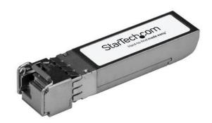
The 10G-SFPP-BXU-ST is a Brocade 10G-SFPP-BXU compatible upstream fiber SFP transceiver which pairs with StarTech.com's 10G-SFPP-BXD-ST. They are designed, programmed and tested to work with 10GBase-BX compatible Brocade switches and routers. The SFP+ transceiver module supports a maximum distance of up to 10 km (6.2 mi) and delivers dependable 10 GbE connectivity over fiber cabling.
