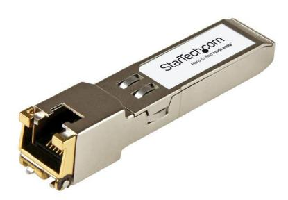
The 10065-ST is an Extreme Networks 10065 compatible copper transceiver module that has been designed, programmed and tested to work with Extreme Networks brand switches and routers. It delivers dependable 1 GbE connectivity over copper cable, for 1000Base-T compliant networks, with a maximum distance of up to 100 m (328 ft).
