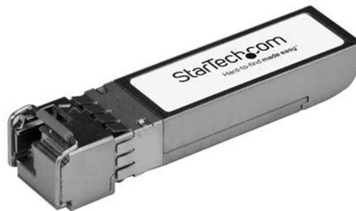
The 10G-SFPP-BXD-ST is a Brocade 10G-SFPP-BXD compatible downstream fiber SFP transceiver which pairs with StarTech.com's 10G-SFPP-BXU-ST. They are designed, programmed and tested to work with 10GBase-BX compatible Brocade switches and routers. The SFP+ transceiver module supports a maximum distance of up to 10 km (6.2 mi) and delivers dependable 10 GbE connectivity over fiber cabling.
