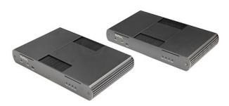
This 4-Port USB 3.0 over Ethernet extender kit includes a transmitter and receiver that enable you to connect four remote USB devices to a local computer up to 330 ft. (100 m) away, using a single standard CAT6a, or CAT7 cable with RJ-45 connectors. For added versatility the USB extender can also extend your Gigabit Ethernet connection to the same remote location.
