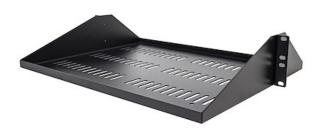
The SHELF-2U-14-CENTER-V lets you add 2U 14 inches (35.6 cm) deep shelf to any 2-post EIA-310 compliant 19-inch rack or cabinet. The shelf is vented to improve airflow and help lower temperatures in your rack.
