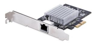
Install this single-port 10GbE PCI Express (PCIe) Network Interface Card (NIC) into a server or computer to enable faster network speeds and enhanced network functionality. This card supports six speeds: 10/5/2.5/1Gbps and 100/10Mbps. The variable speeds permit access to legacy hardware. Alternatively, the 10GBASE-T and NBASE-T capabilities ensure compatibility with the latest network switches and network access points manufactured by Cisco, HPE, and Aruba.
