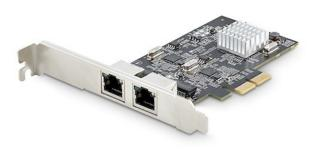
This dual-port 2.5 GbE network interface card (NIC) features an Intel I225-V chipset with Intel vPro technology, to enhance performance and data integrity across two 2.5G ethernet connections. The variable multispeed options (2.5/1Gbps and 100/10Mbps) enable support for both new and legacy network hardware. Utilize existing Cat5e or CAT6 cabling infrastructure while adding NBASE-T (802.3bz) compatibility for seamless integration.
