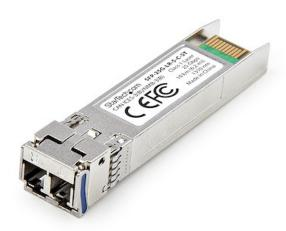
This fiber optic transceiver is the direct equivalent to Cisco SFP-25G-LR-S for 25Gbps connectivity up to 10km (6.2mi) over LC-terminated Single Mode Fiber (SMF) cable. The optical module has been programmed and tested for seamless integration with Cisco switches and routers to ensure compatibility and reliability.
