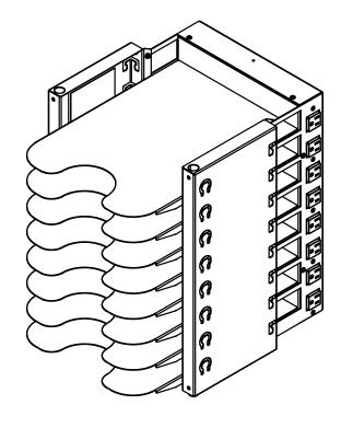
Use the Collectiv8<sup>™</sup> Charging Pillar to store and charge up to 8 devices (most tablets, Chromebooks<sup>™</sup>, and notebooks). Wiring slots keep cords organized and speed wiring to each bay. The Collectiv8 Pillar's small footprint covers less counter space, and is made with powder-coated steel for durability.
