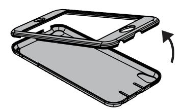
**2.** Place case front on flat surface face down, push down on back frame all around edges to engage snaps.
